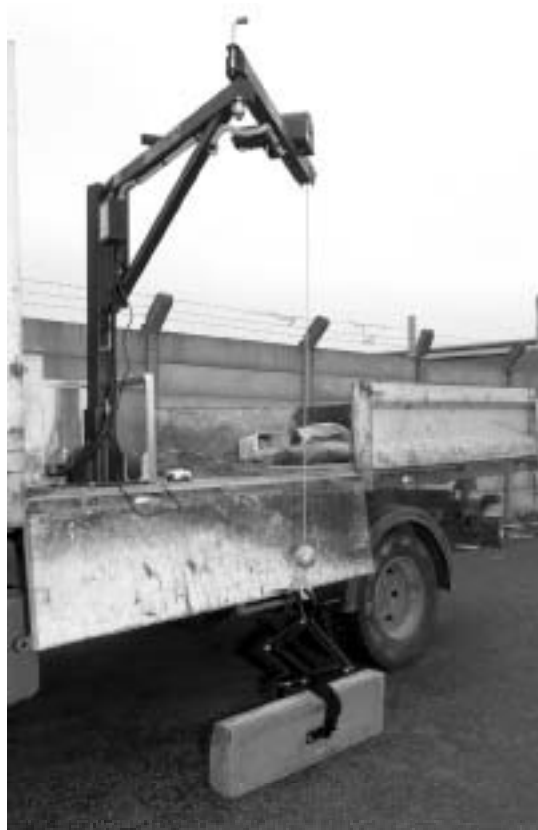
Figure 2 Vehicle-mounted crane and mechanical grab
